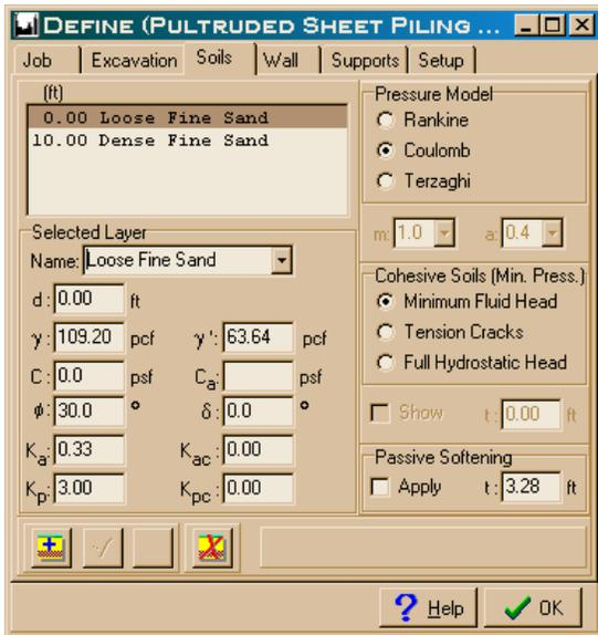
Step 3. Input the soils data. From ground level to the excavation depth of 10', the soil is loose fine sand; below this 10' mark, it becomes dense fine sand. In this example the Coulomb theory of modeling lateral earth pressure is chosen as an option in Pile Bucks SPW 911 V2 sheet piling retaining wall software program. Alternatives would be the Rankine or Terzaghi pressure models or hand calculations.
