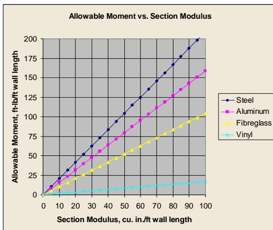
The chart to the left<sup>1</sup> shows the relationship between the section modulus and the allowable bending moment for a selection of sheet pile manufactured in (4) different materials, using the formula above. It can be seen first that, for a section with the same section modulus, sections manufactured from pultruded fiberglass have a higher allowable bending moment (by a factor of more than six) than comparable vinyl sections.
