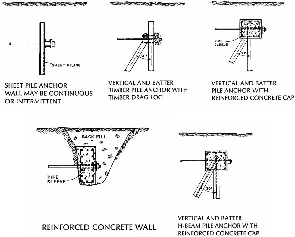
(5) TYPICAL SHEET PILING BULKHEAD ANCHORING METHODS UTILIZING A CONVENTIONAL GALVANIZED TIE-ROD.
